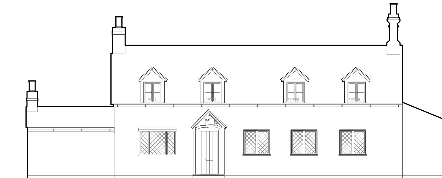
Existing FRONT Elevation
