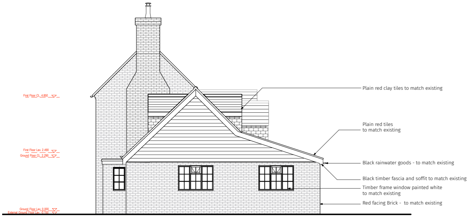
PROPOSED SIDE (EAST) ELEVATION
