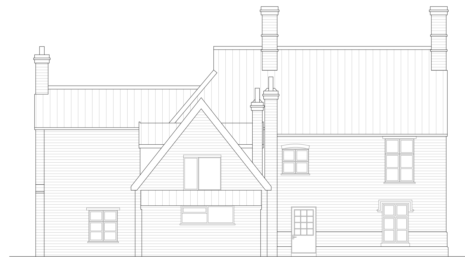
Existing South Elevation @ 1:100
