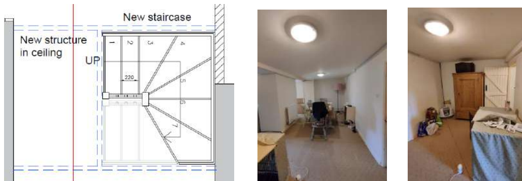
Figure 113 Proposed floor plan of the new staircase in Games Room Figures 114 & 115 Images of existing games room
