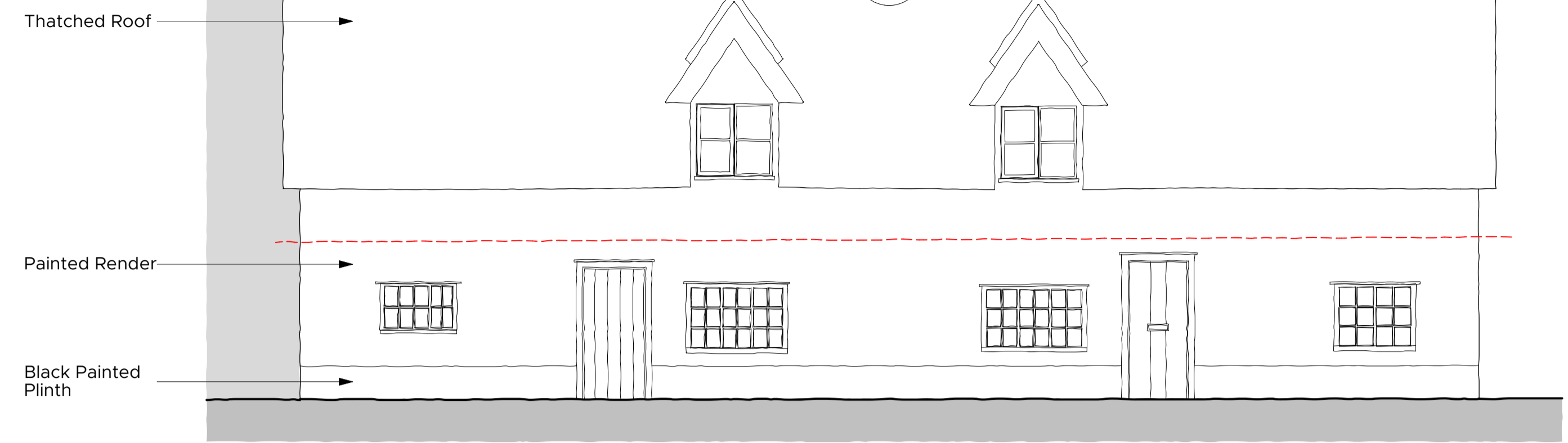
EXISTING NORTH ELEVATION (FRONT) Scale 1:50
