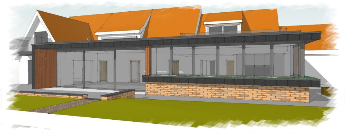
Oblique view of rear façade showing extent of glazing and overhangs
