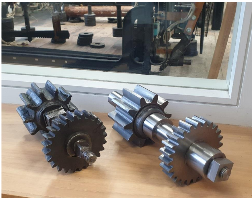
Below: Newly produced sluice gearing assembly (right) to replace worn original (left) -WSM
