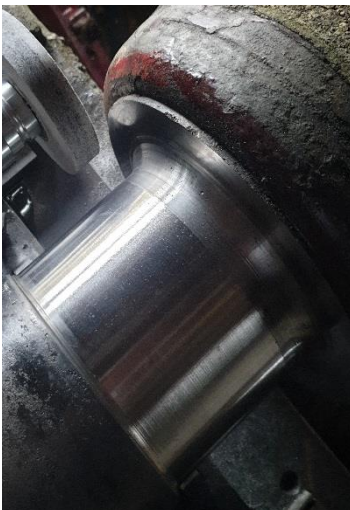
Left: Waterwheel axle after machining in situ. A process that could only have been achieved after design and production of complex bespoke tooling.
