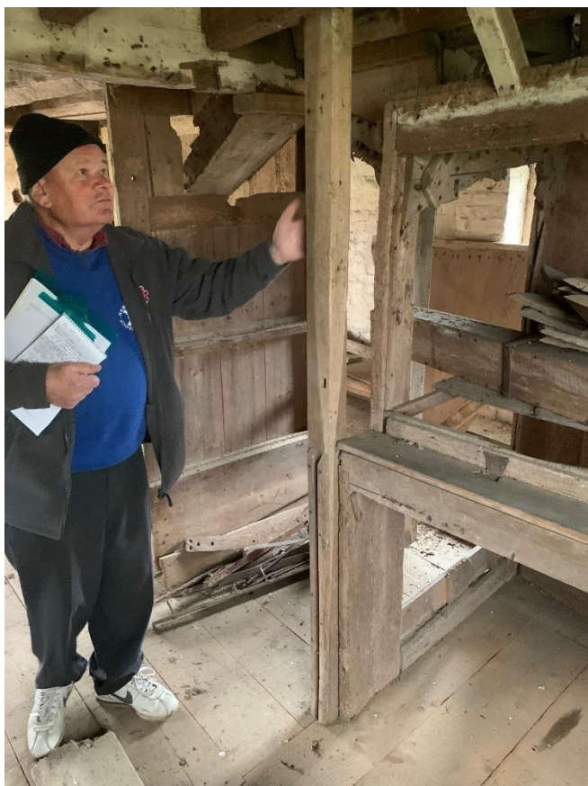
David Plunkett of Hampshire Mills Group (HMG) standing by the post attached to the flour dresser. The dresser separates the whole meal into bran and unbleached white flour.
