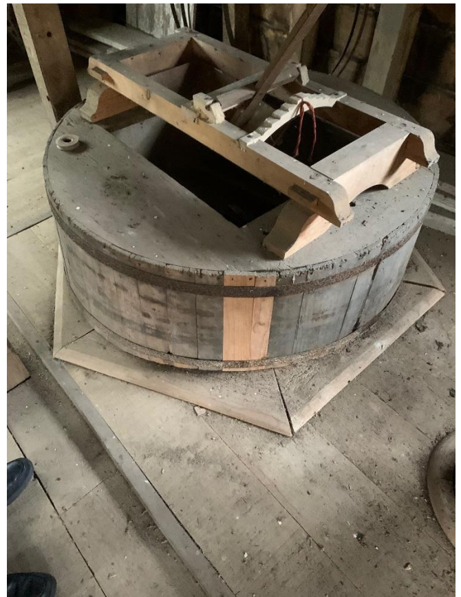
The Damsel, Horse, and Shoe containing the Millstones. This is where the grain would have been fed from a hopper into the shoe, which is vibrated by the damsel, shaking grain into the centre of the runner stone. - All to be retained and refurbished.
