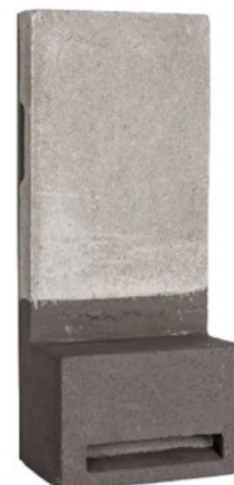
Bat brick (26mm hole) to be built as high as possible on the eastern elevation of new section.
