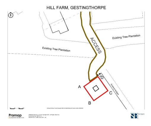
Boundaries A-B, B-C and C-D will be fenced with stock netting fencing with a single line of barbed wire over. Stock netting will be HT13/122/7.5 CLASSIC HORSE HIGH TENSILE STEEL FENCE NETTING which has a height of 122cm. <a href="https://www.clarkesofwalsham.co.uk/product/ht13-122-7-5-classic-horse-high-tensile-steel-fence-netting-50mtr-roll/">https://www.clarkesofwalsham.co.uk/product/ht13-122-7-5-classic-horse-high-tensile-steel-fence-netting-50mtr-roll/</a>
