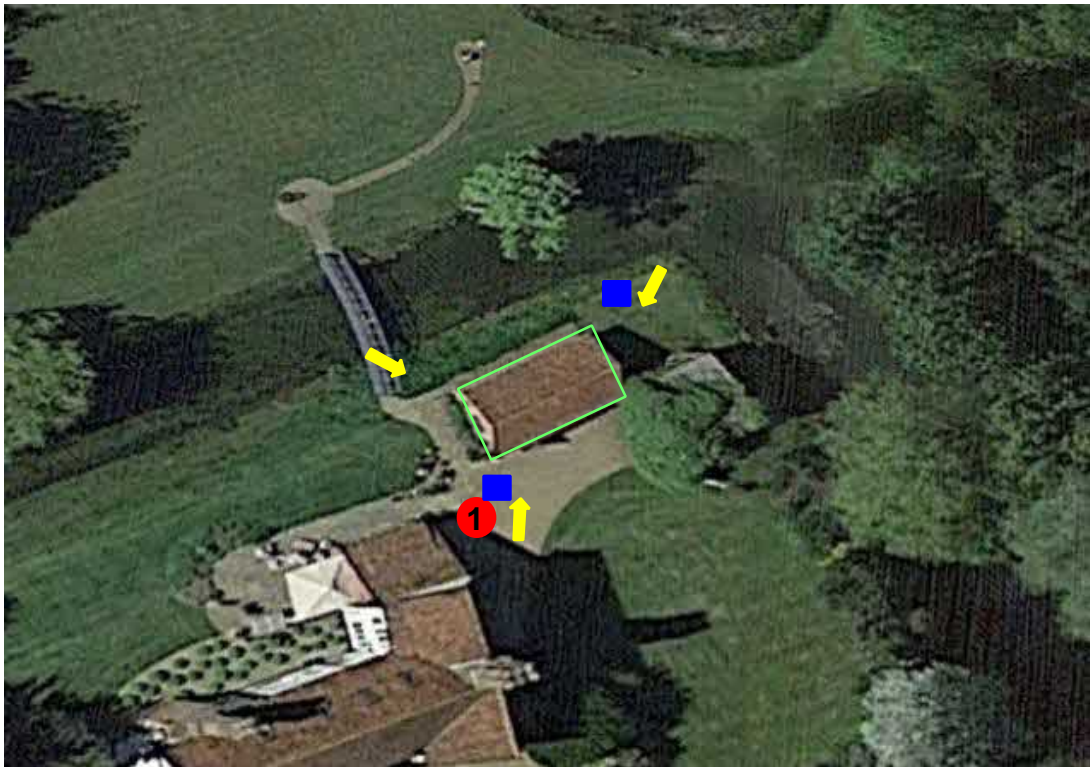
Fig 3: Surveyed building outlined in green. Surveyor location indicated by red circle; camera - yellow arrows, detectors - blue squares.
