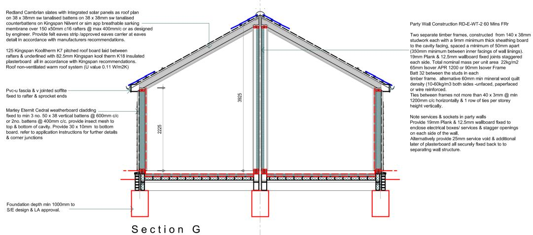
studwork each with a 9mm minimum thick sheathing board to the cavity facing, spaced a minimum of 50mm apart (350mm minimum between inner facings of wall linings). 19mm Plank & 12.5mm wallboard fixed joints staggered each side. Total nominal mass per unit area 22kg/m2 timber frame. alternative 60mm min mineral wool quilt density (10-60kg/m3 both sides -unfaced, paperfaced or wire reinforced. Ties between frames not more than 40 x 3mm @ min
