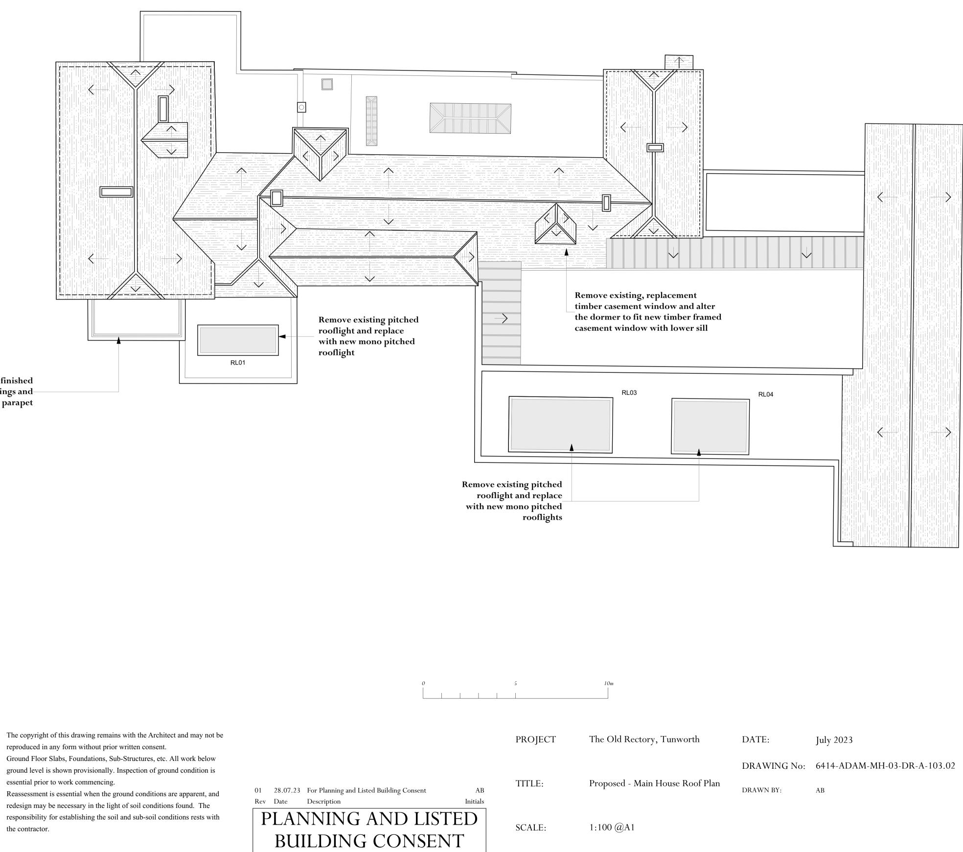
New paint finished metal railings andhandrail to parapet
