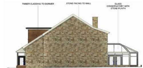
North West Elevation
