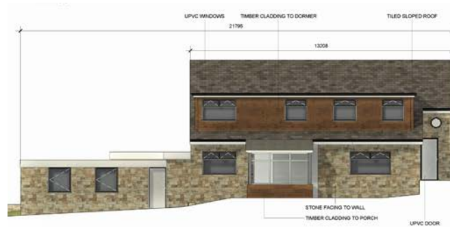
South West Elevation
