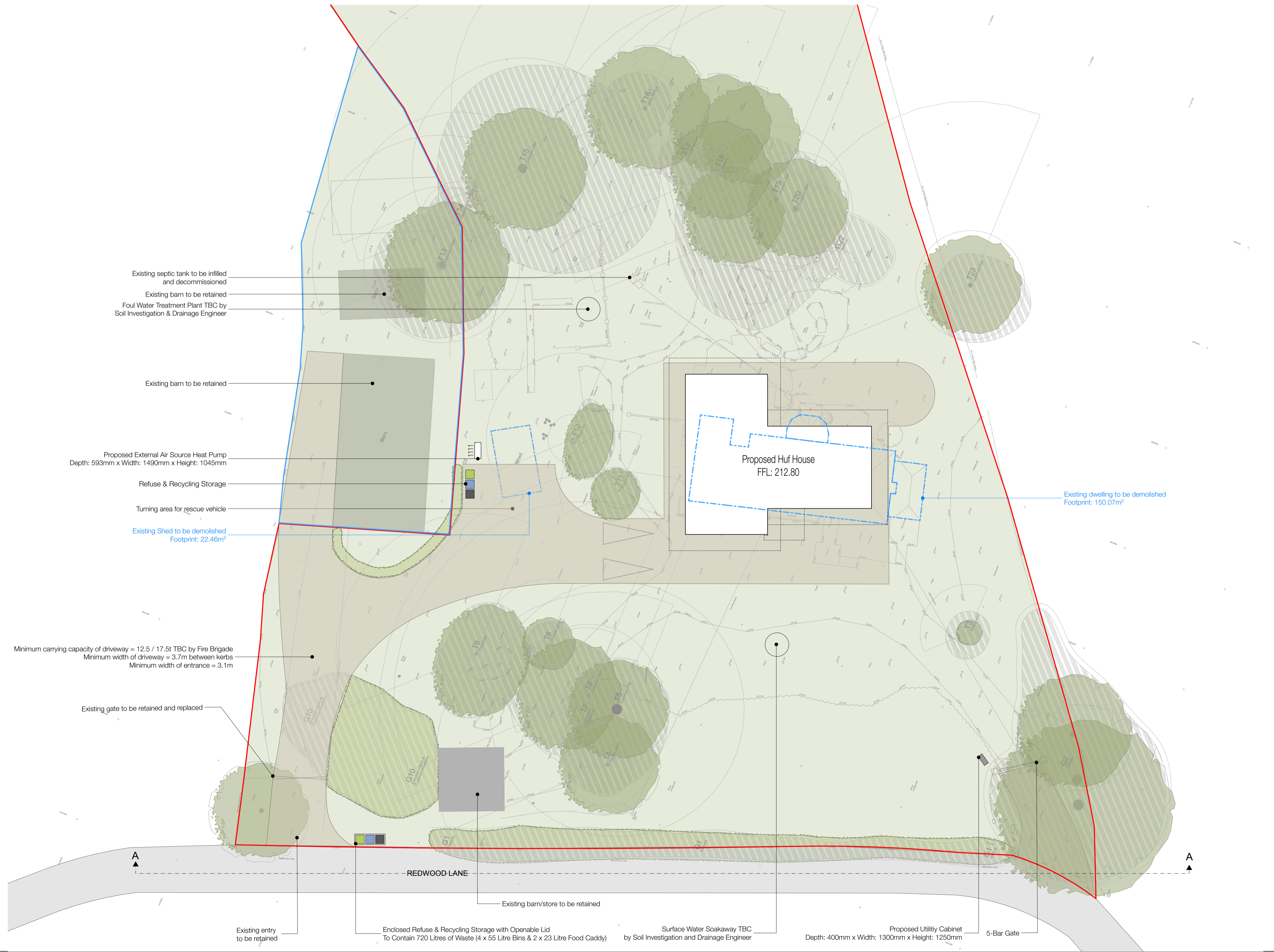
Minimum carrying capacity of driveway = 12.5 / 17.5t TBC by Fire Brigade Minimum width of driveway = 3.7m between kerbs Minimum width of entrance = 3.1m
