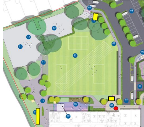
LONG TERM CYCLE PARKING SHOWN YELLOW AND SHORT-TERM CYCLE PARKING LOCATION SHOWN IN RED
