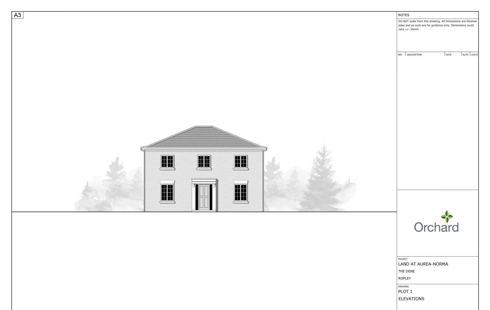
PLOT 1 - FRONT ELEVATION MATERIALS: RED BRICK WITH SLATE ROOF
