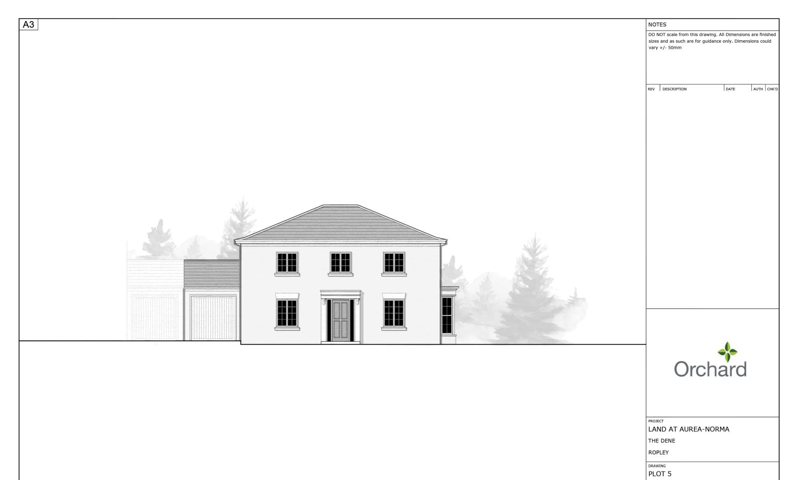
PLOT 5 - FRONT ELEVATION MATERIALS: RENDERED WITH SLATE ROOF
