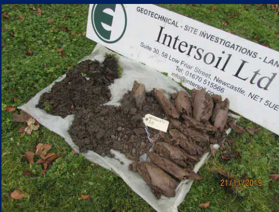
Typical made ground arisings to left and natural clay to right (A3)
