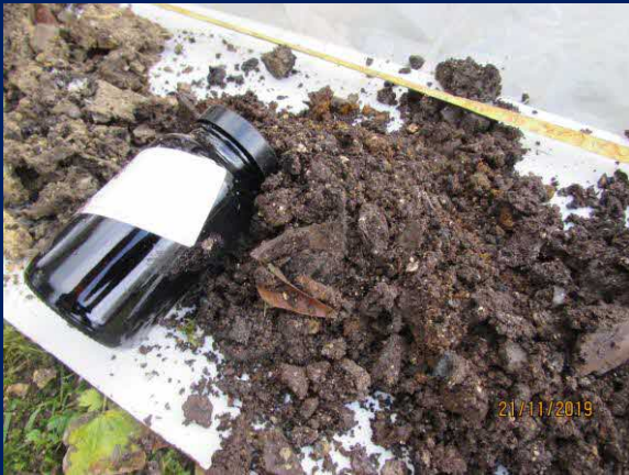
Typical ash and clinker arisings from one of the hand augered holes (A1)
