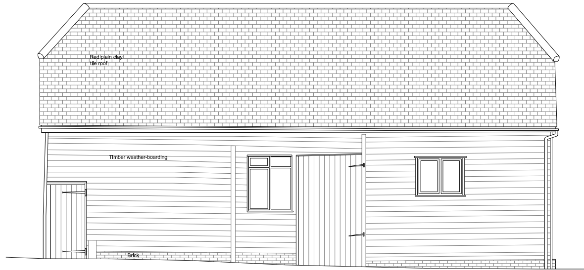
Barn K Existing East Elevation
