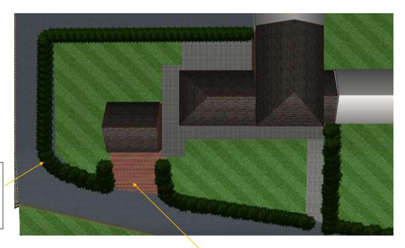
This corner too tight for vehicle accessing properties to rear, moving wall in to assist with neighbours access.
