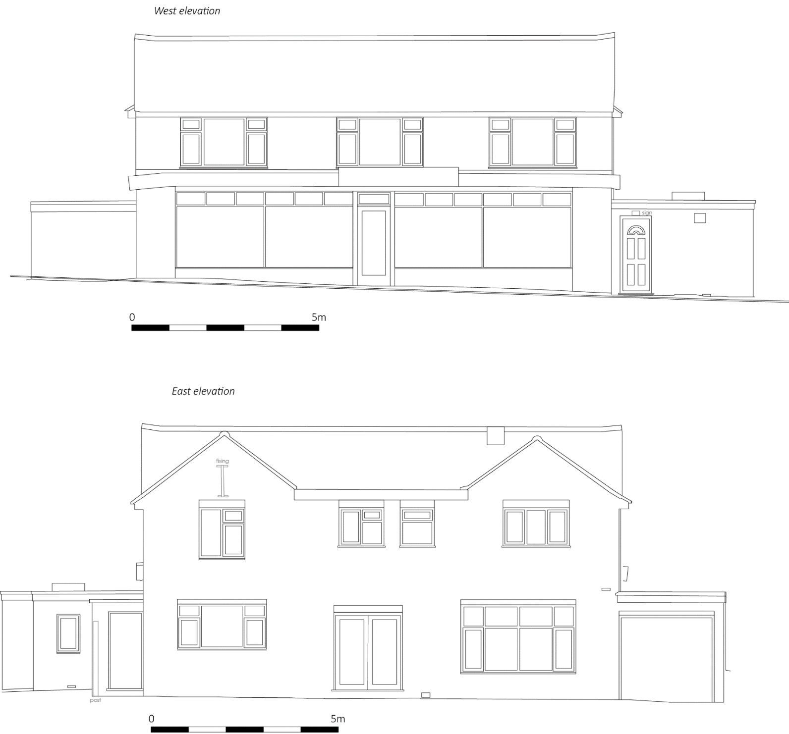
Figure 8: Front building, front and rear elevations (scale 1:100)
