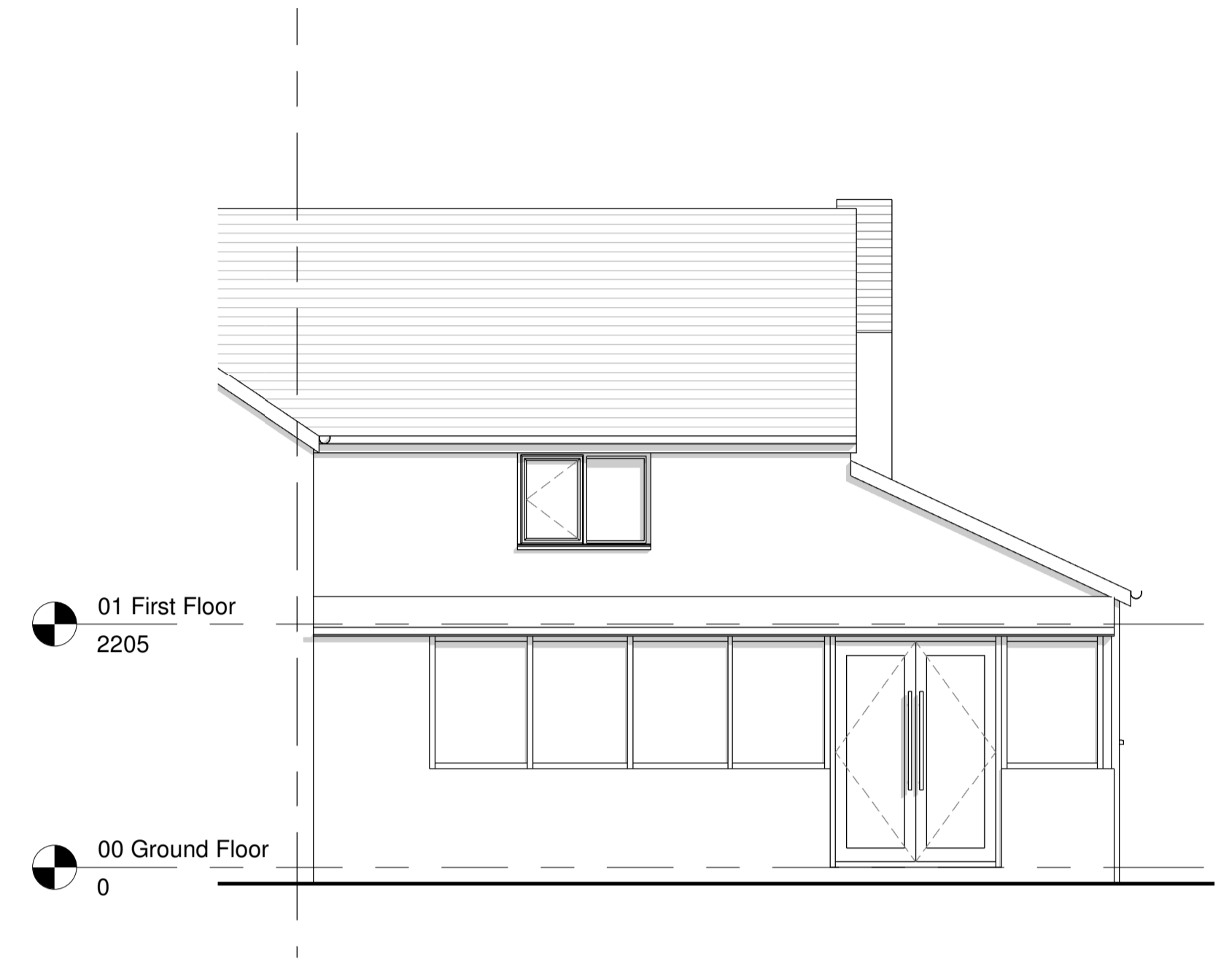
Existing West Elevation 1 : 50
