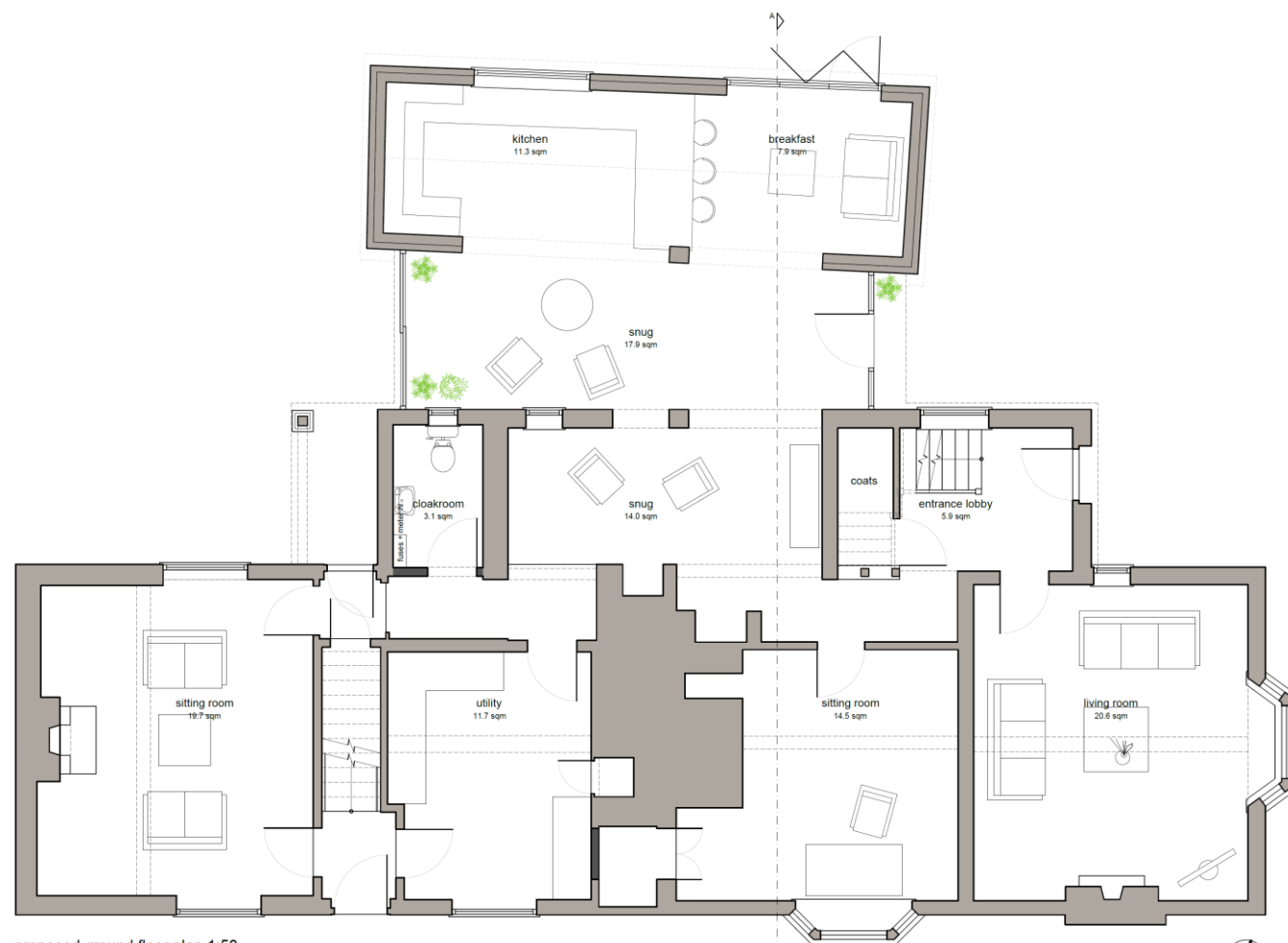
proposed ground floor plan 1:50 Ground Floor Gross Internal Area = 158.3 sqm [1703 sqft] Total Gross Internal Area = 254.4 sqm [2737 sqft]
