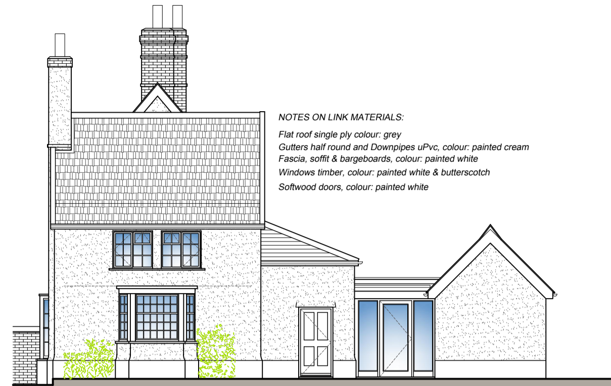
proposed north-east elevation 1:100
