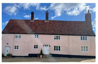
The main part of the house is timber framed and dates from c.1580, the house was extended within 50 years of the original build (you can see the step down in the sole plate of this part of the house).
