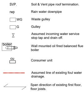
Soil & Vent pipe roof termination. Rain water downpipe Waste gulley Gulley Assumed incoming water service stop tap and drain off. Wall mounted oil fired balanced flue boiler Consumer unit Assumed line of existing foul water
