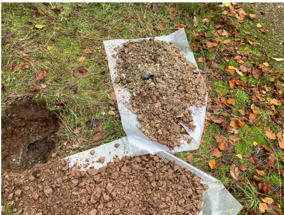
Figure 6-2: Made Ground in HP03
