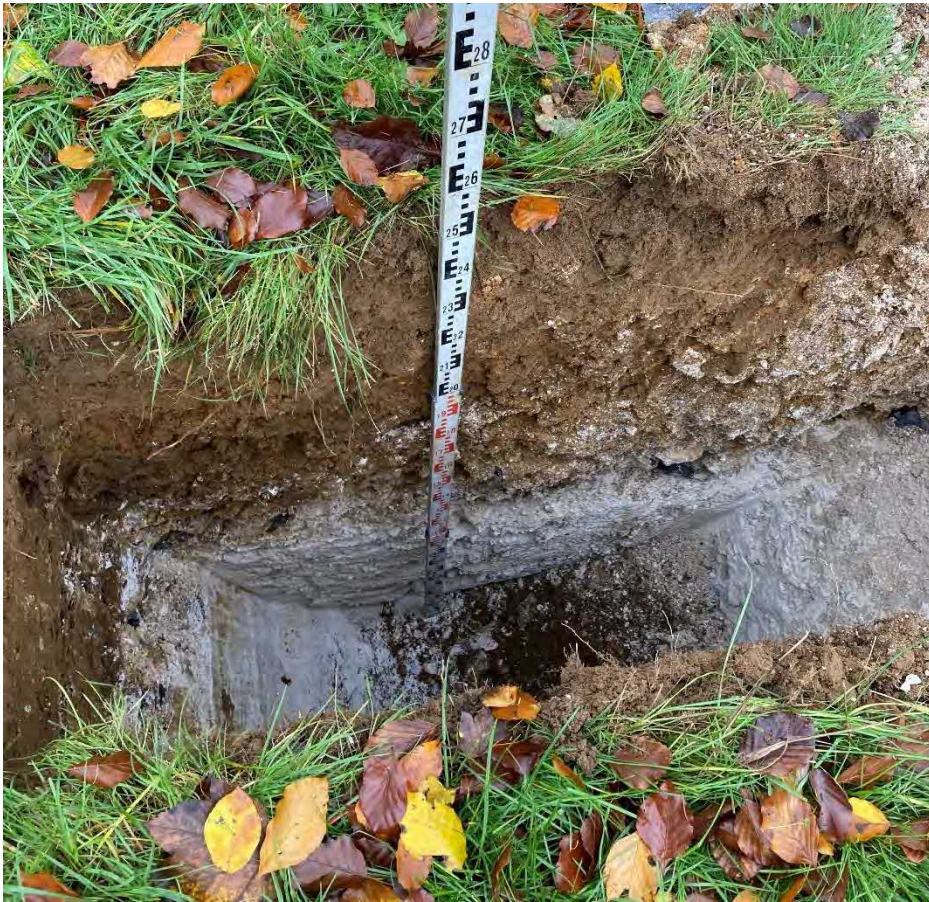
Figure 6-1: Topsoil within TP15
