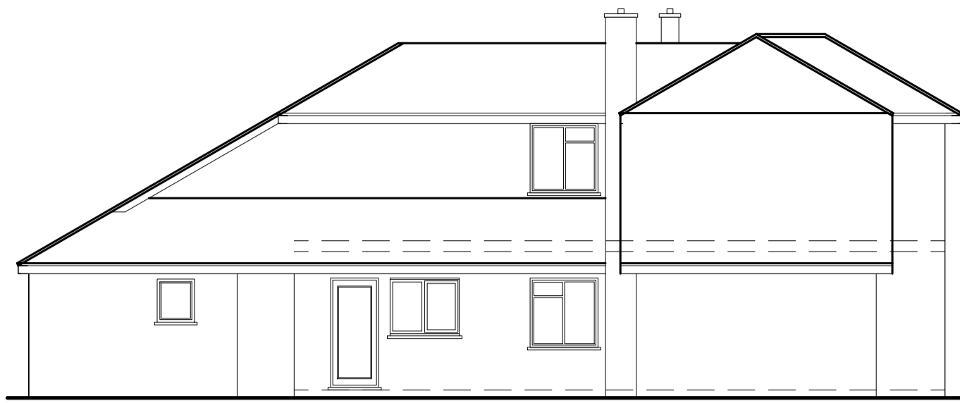
Existing Rear Elevation
