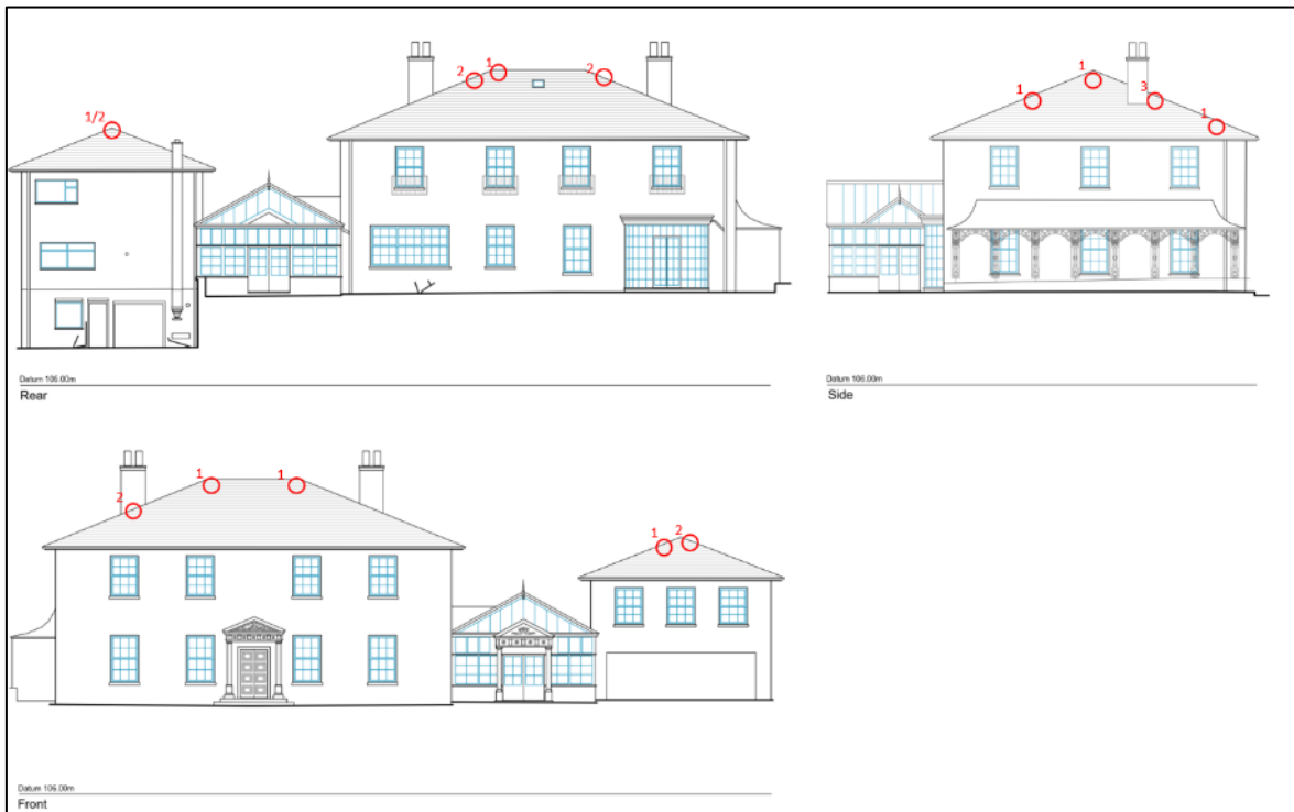
Figure 20: Diagram depicting bat PRF locations. 1=lifted tiles, 2=Gap underneath flashing and 3=bow in roof exposing crevices underneath tiles
