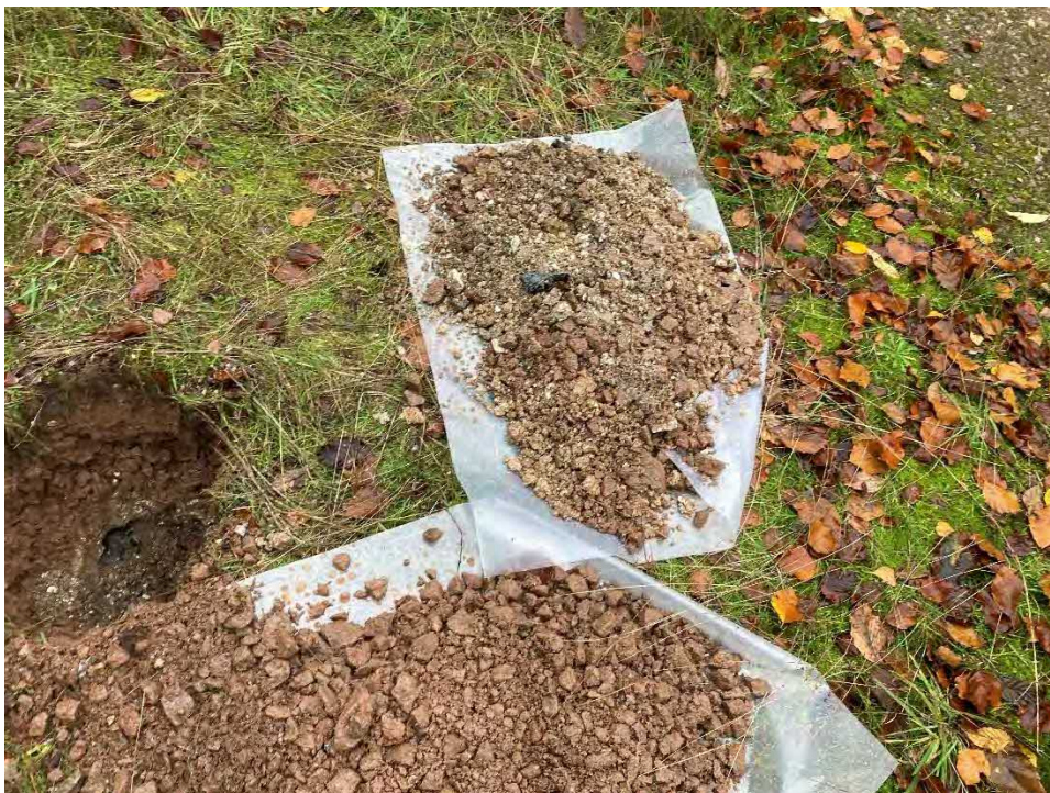
Figure 6-2: Made Ground in HP03
