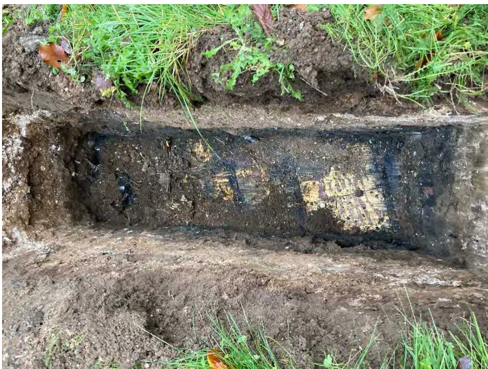
Figure 6-3: Made Ground in TP04
