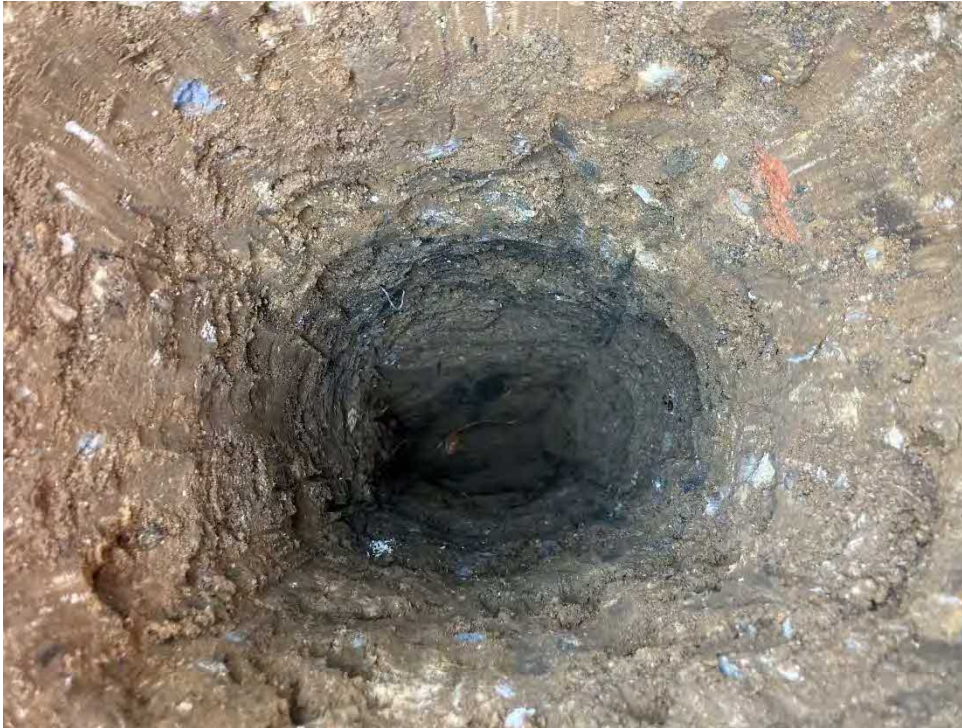
Figure 6-4: Made Ground in HP09 (raised/bunded area to the northeast)
