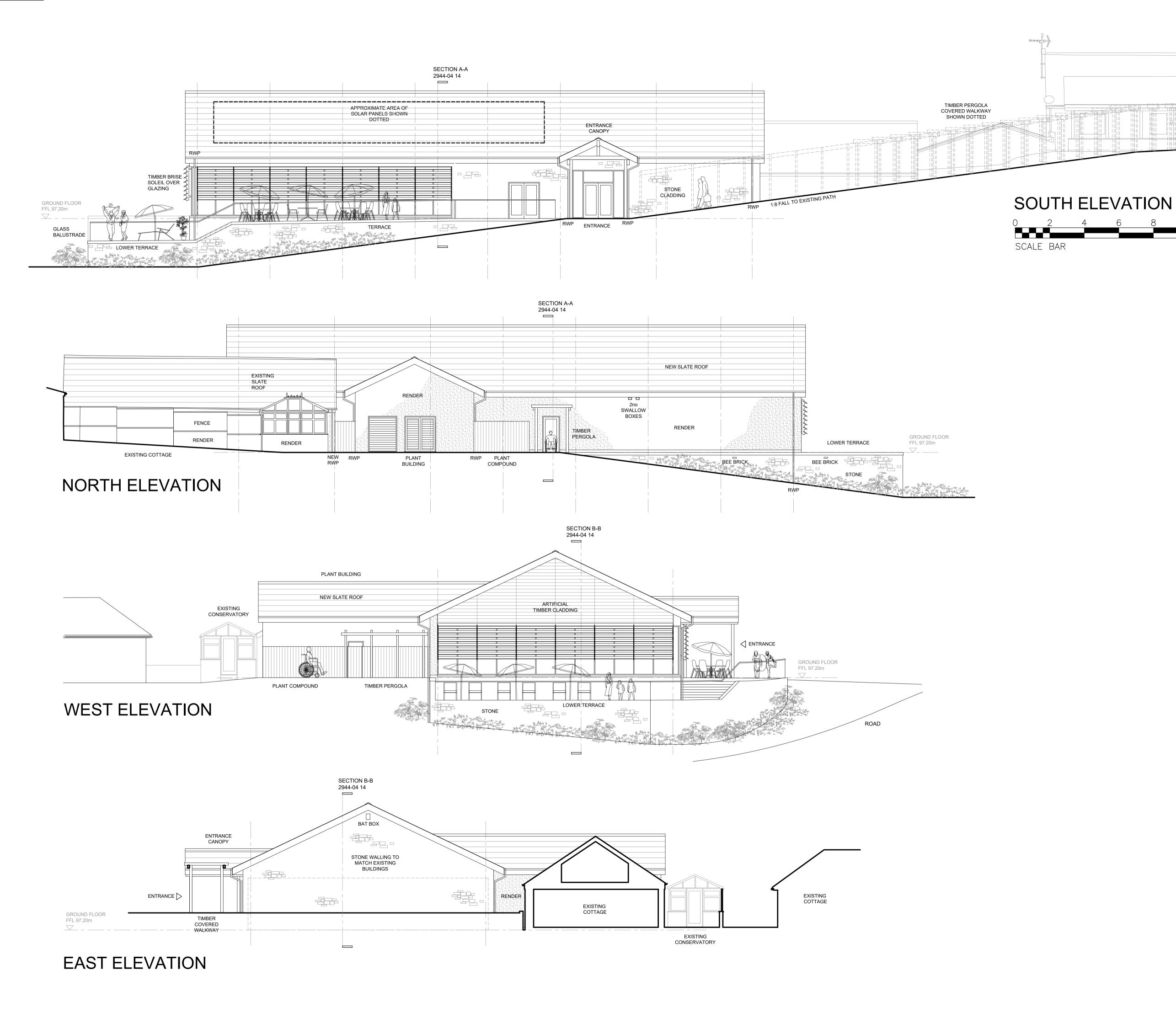
PLANT ROOM AND PERGOLAS ALTERED. RWP MOVED. SLIDING DOOR CHANGED TO DOUBLE DOOR. ROOFLIGHTS REMOVED. 25.07.23 SWALLOW BOXES, BEE BRICKS AND BAT BOX ENTRANCE CANOPY GLASS ADDED. RIDGE AND 14.07.23
