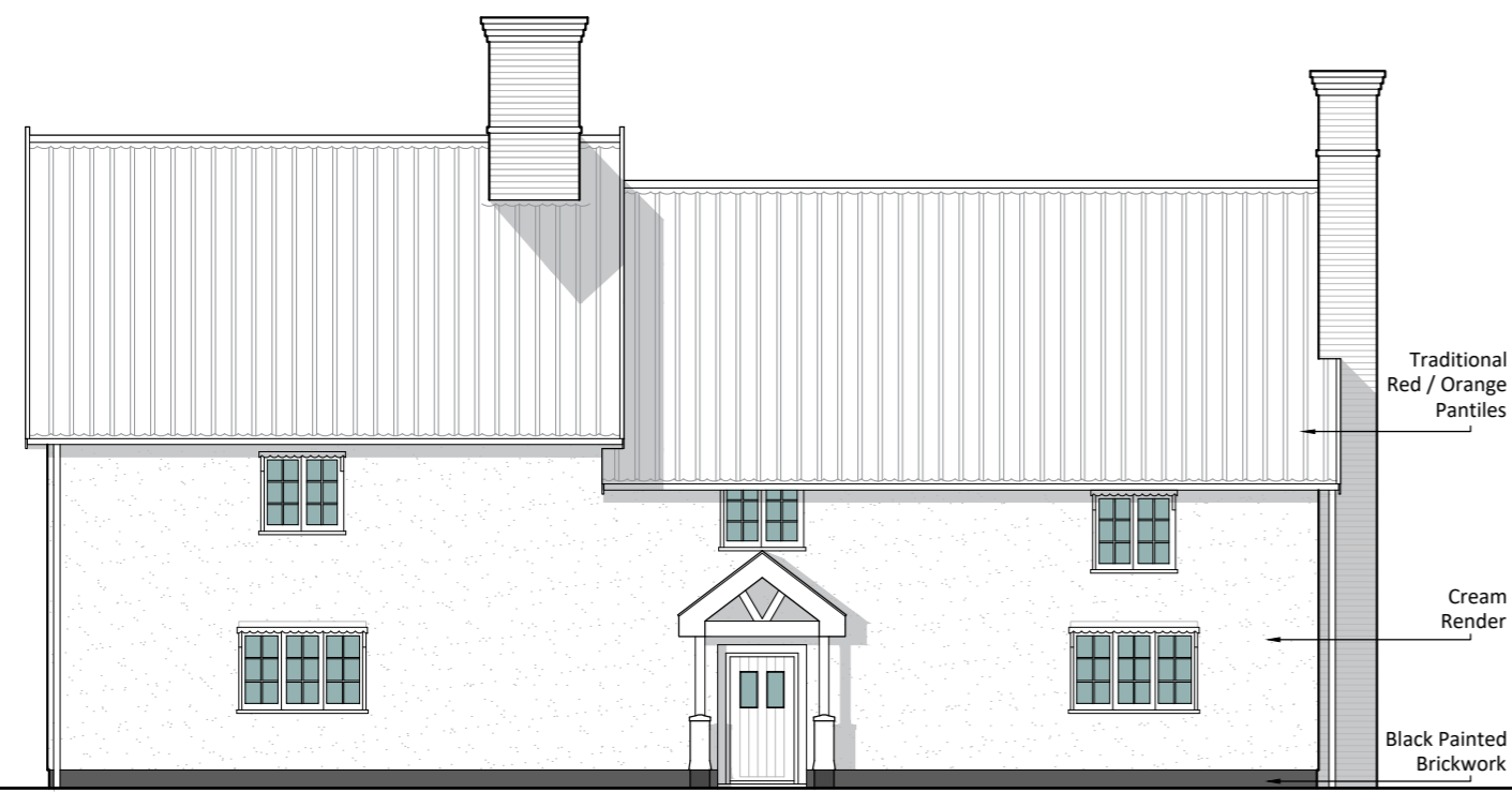
Existing South Elevation 1:100
