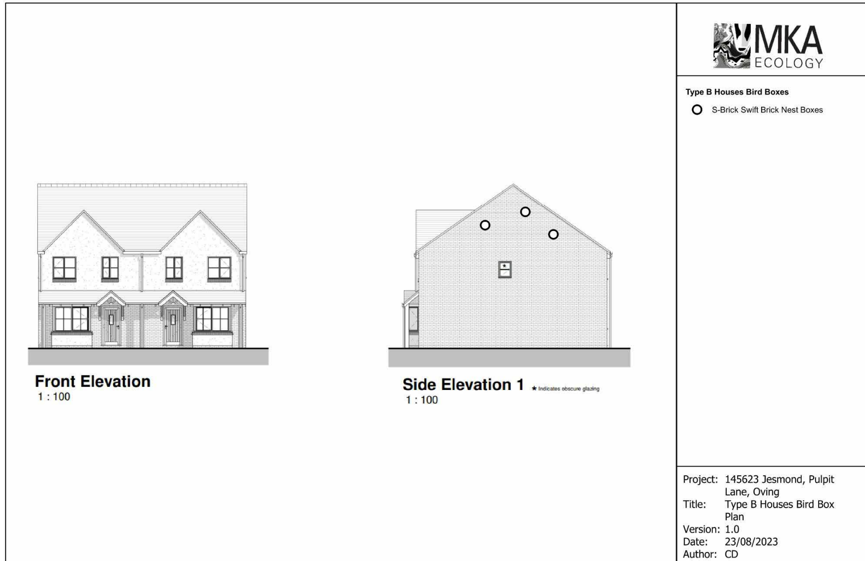
Figure 5: Proposed bird box plan for Type B Houses at Jesmond, Pulpit Lane, Oving
