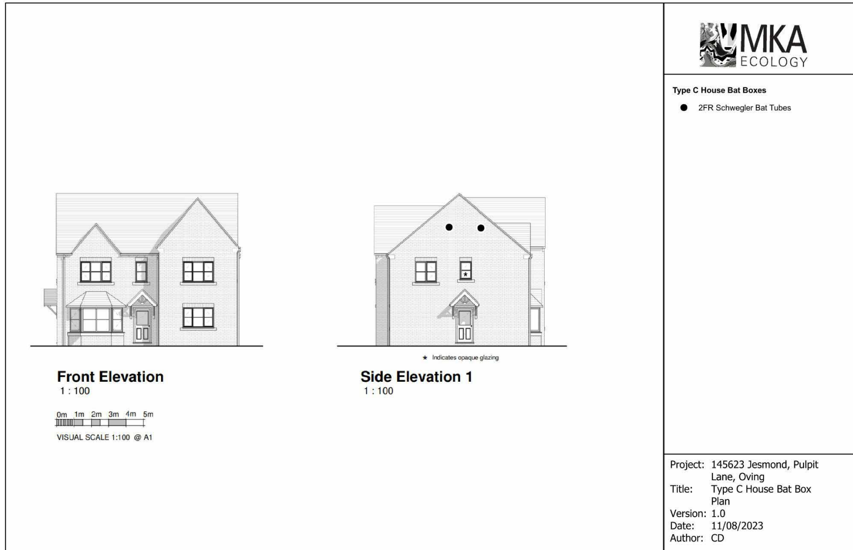
Figure 6: Proposed bat box plan for Type C House at Jesmond, Pulpit Lane, Oving
