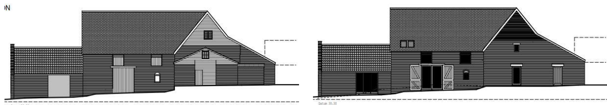
Left: Existing E elevation, scale 1 : 100 @ A1 (Patrick Allen & Associates Architects drawing 4411-03A); Right: Proposed E elevation, scale 1 : 100 @ A1 (Patrick Allen & Associates Architects drawing 4411-07)
