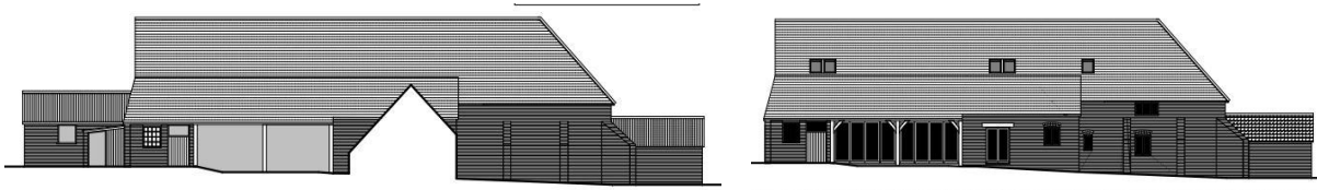
Left: Existing S elevation, scale 1 : 100 @ A1 (Patrick Allen & Associates Architects drawing 4411-03A); Right: Proposed S elevation, scale 1 : 100 @ A1 (Patrick Allen & Associates Architects drawing 4411-07)
