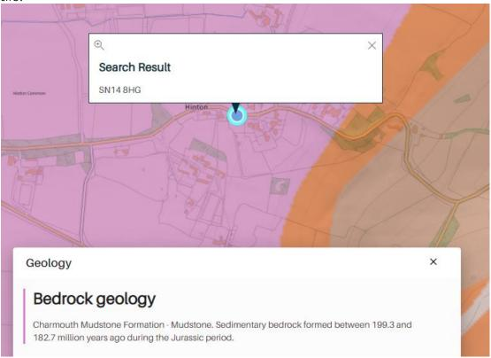
Review of local boreholes for the surrounding works available on BGS suggest the shallow substructure likely to be encountered to be of Firm Grey/Green Clay with small clusters of limestone and siltstone bands close to the surface level.
