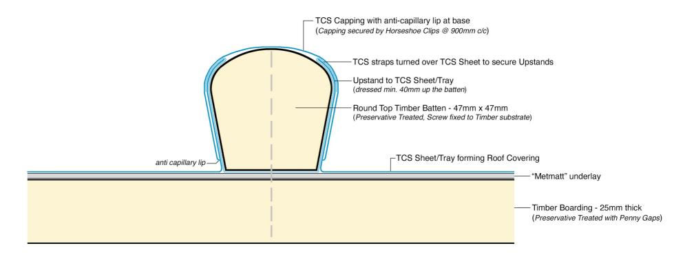
TCS Grade, Thickness, Finish and other details to be as stated in the Relevant Project Specification TCS shall generally be grade 316 or K44 grade, 0.5mm thick (possibly 0.4mm for detail work) with "Uginox Patina" or similar finish
