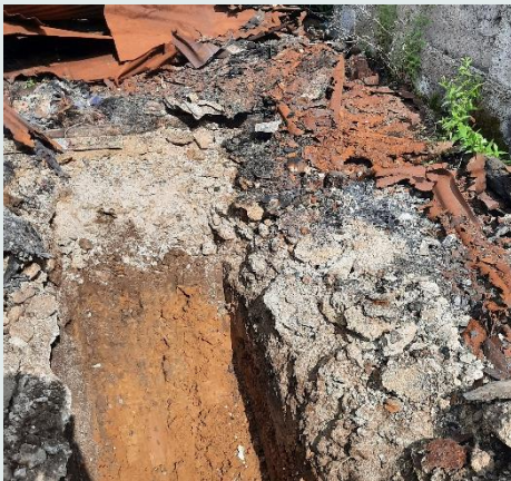
Made Ground of gravelly ashy sand in TP2
