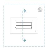
Weather / rot proofed chassis (glulam / engineered timber) placed on levelling shims (not shown) upon hard surface. No foundation / physical connection to ground beneath.
