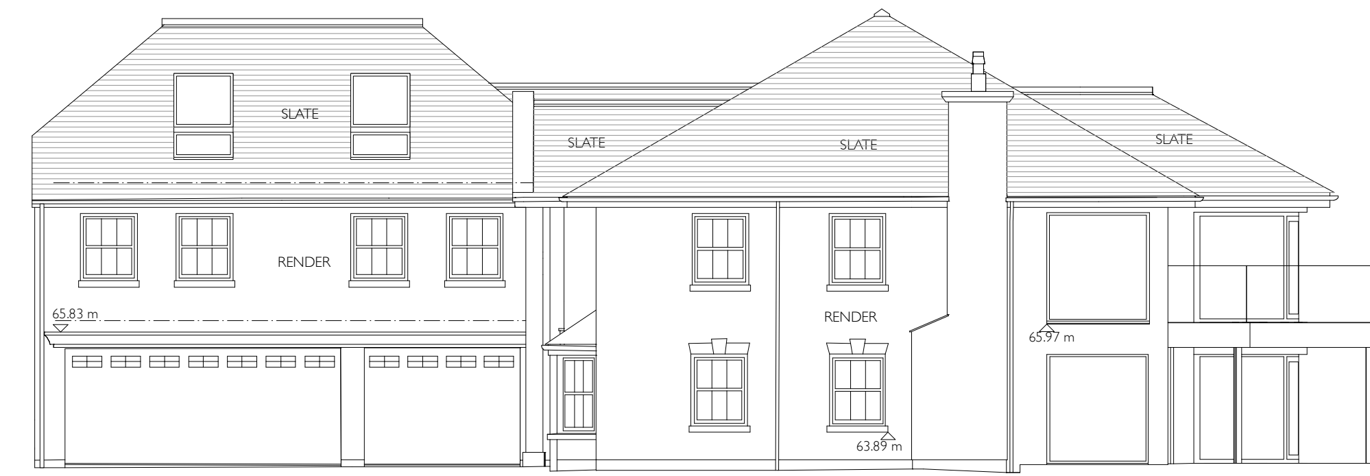
SOUTH WEST ELEVATION
