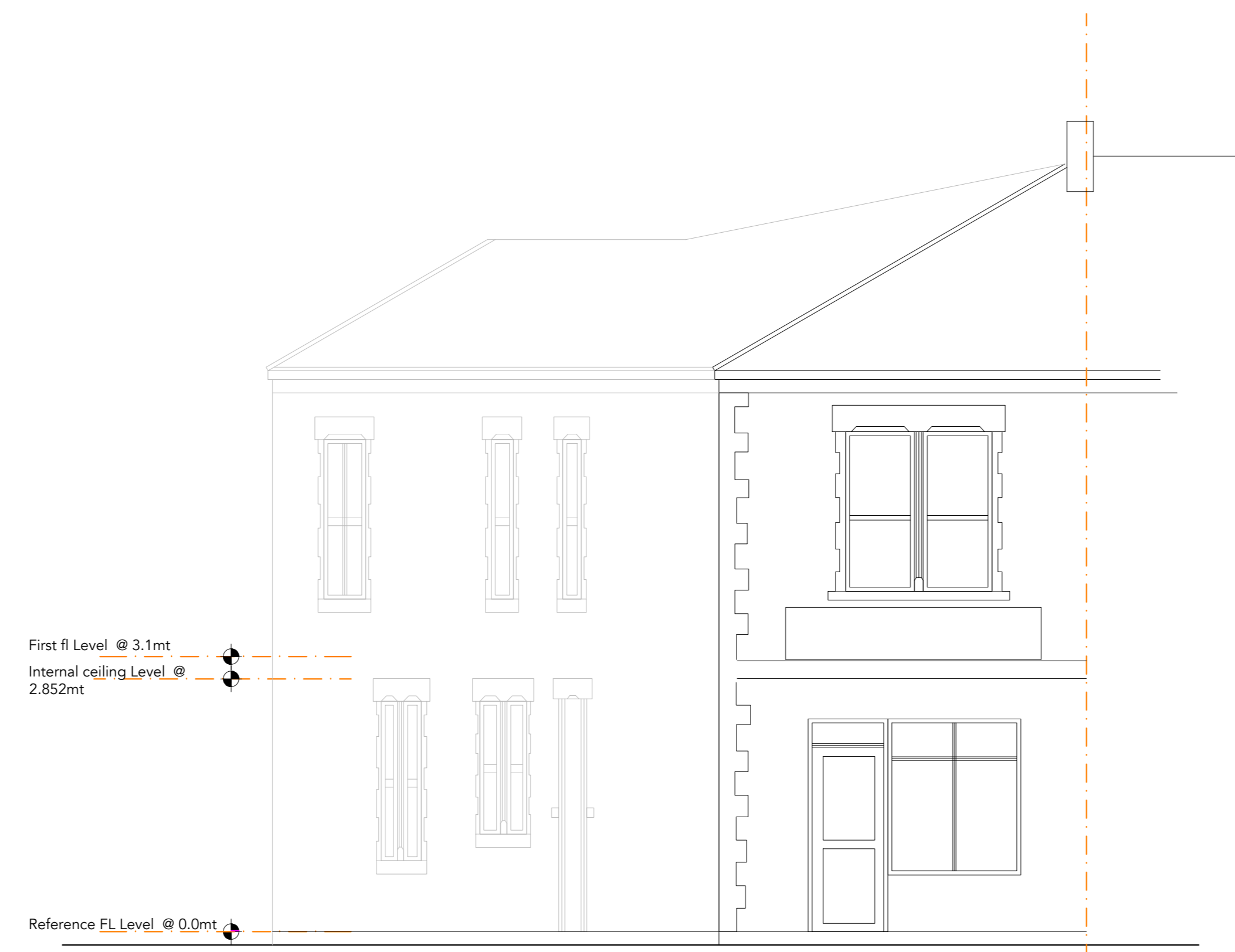
EXISTING FRONT ELEVATION A
