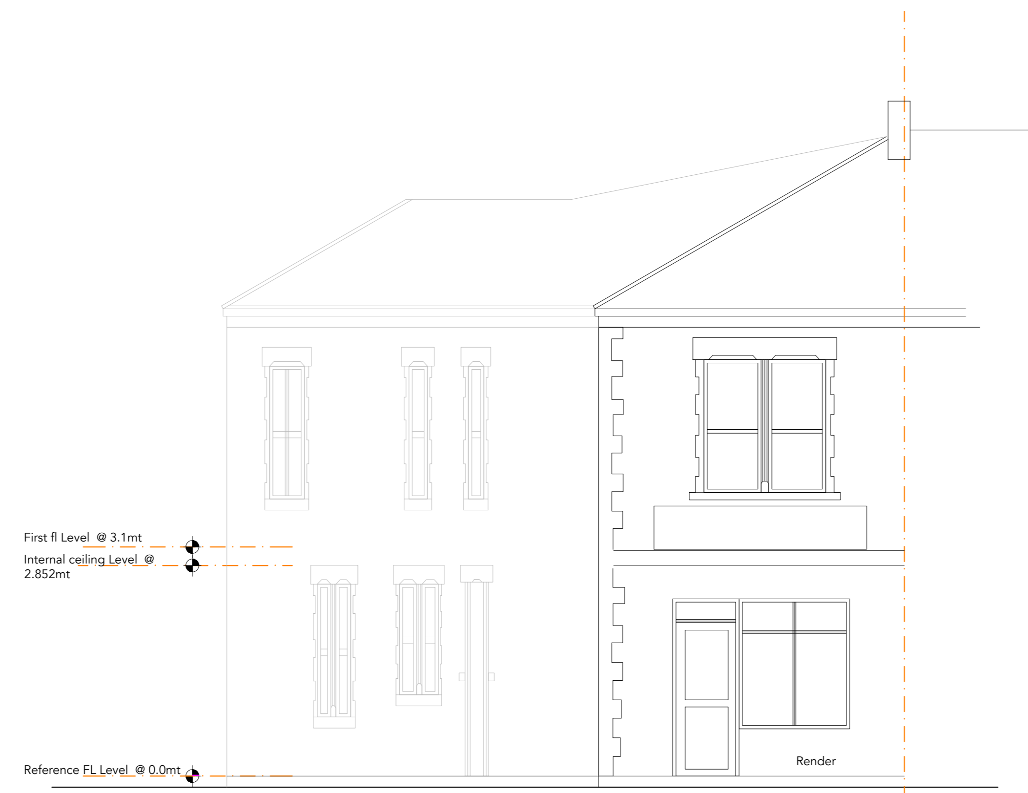
PROPOSED FRONT ELEVATION A NO CHANGE
