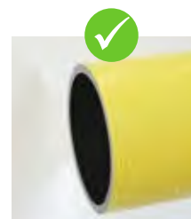
Correct pipe preparation for electrofusion
