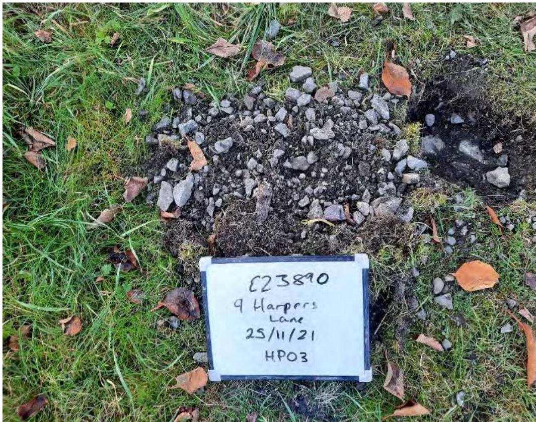
Photo 6: Hand Pit Spoil
