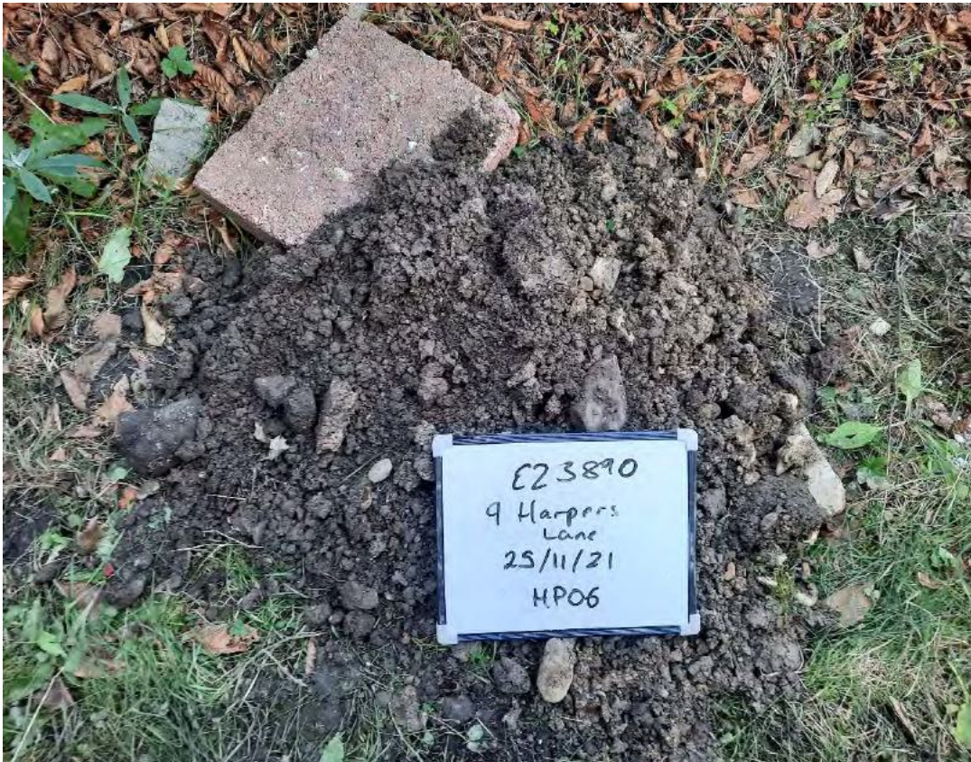
Photo 12: Hand Pit HP06 Spoil
