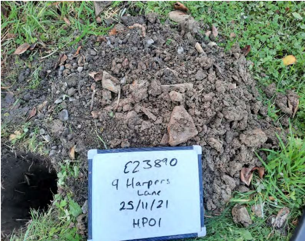
Photo 2: Hand Pit HP01 Spoil
