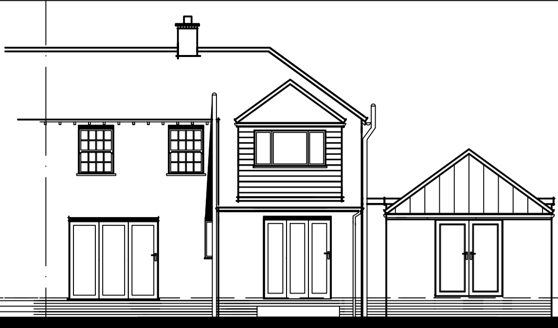
PROPOSED REAR ELEVATION 1:100
