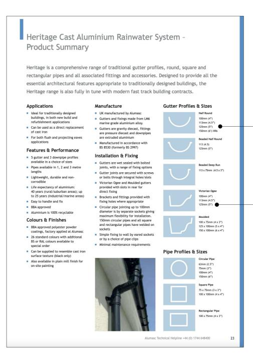
Alumasc Extract Indicating Gutter Profiles and Downpipe Profiles
