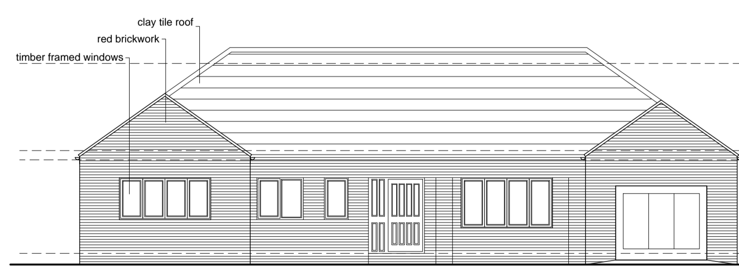
North Existing Elevations - 1:100
