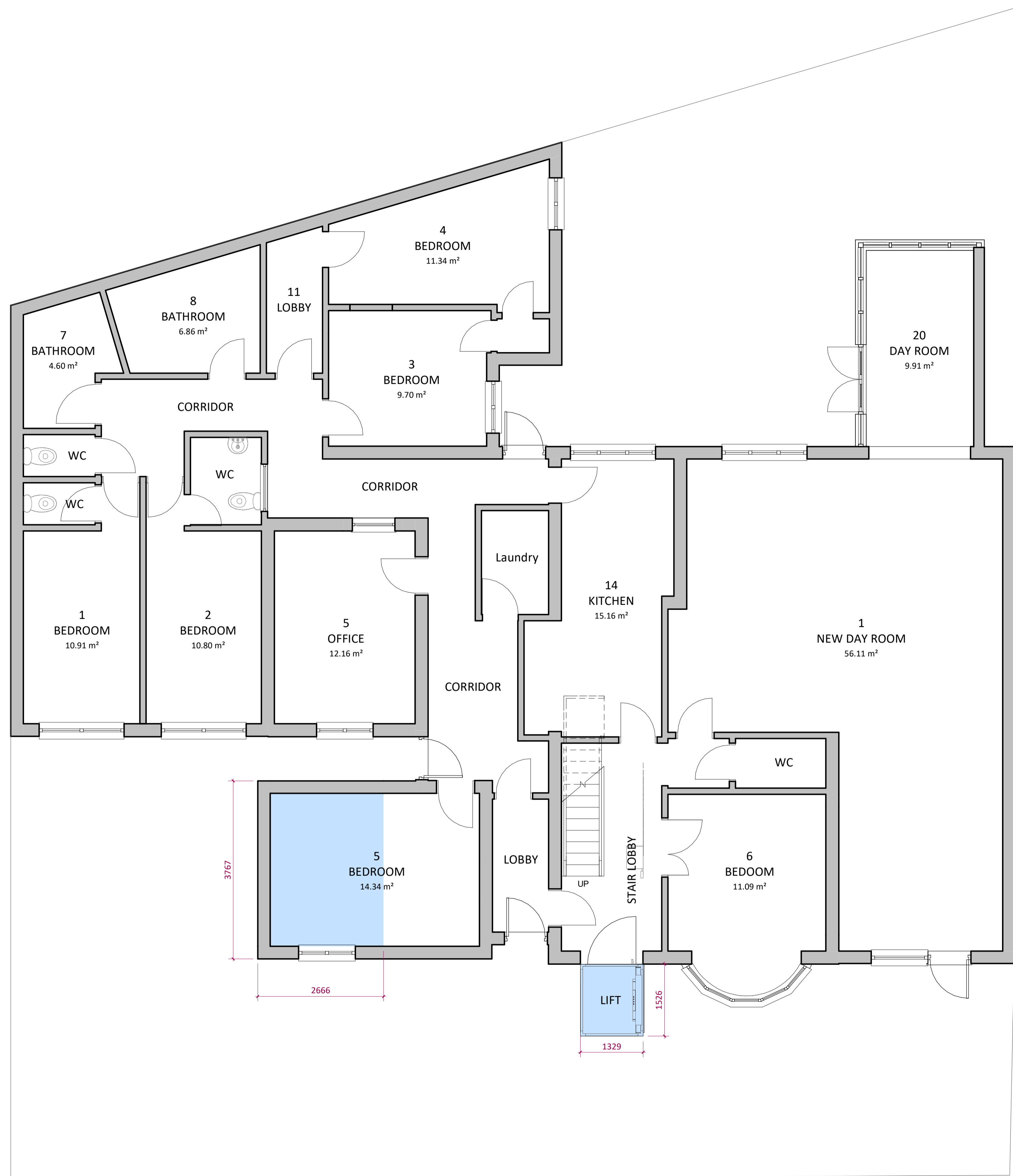
1 PROPOSED - GROUND FLOOR PLAN - COMPLETE 1 : 50
