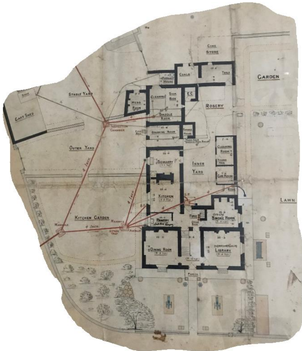
Figure 11 – Extract from “Plan shewing Drainage and Water Supply executed for Major Charles Hall”, 1906 showing the ground floor plan of Lamyatt Lodge
