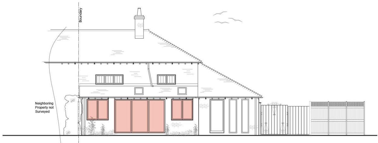
South East Elevation as proposed, highlighting the proposed new door and windows.
