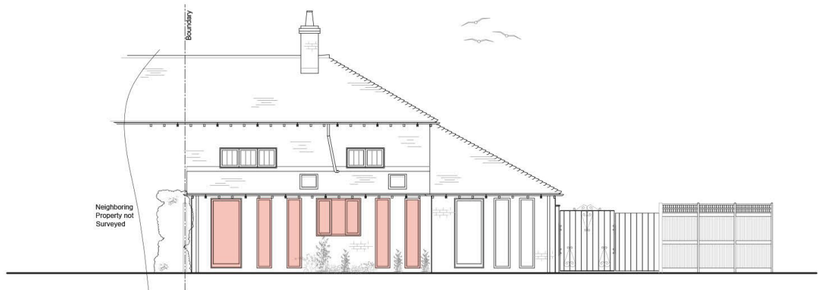
South East Elevation as existing showing modern door and windows proposed to be removed.
